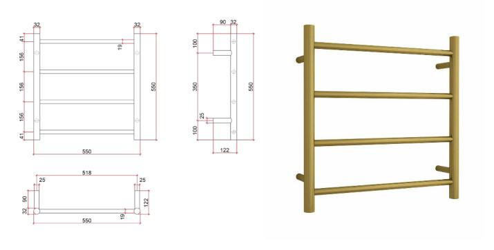
Note: All dimensions are in millimeters (mm)
